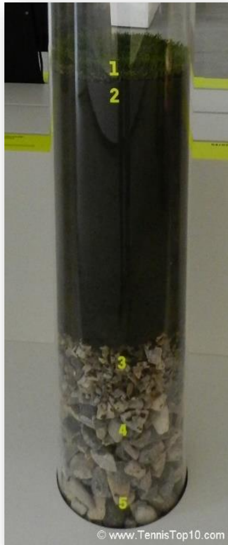
Figure 10 Composition of the Wimbledon courts
